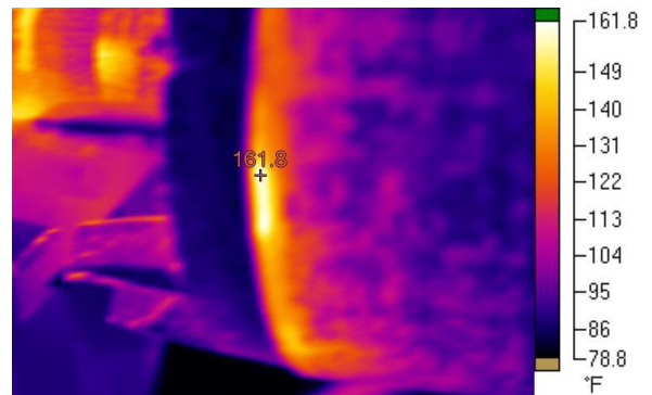
The infrared pictured above shows the hot spot discovered during the core test.
