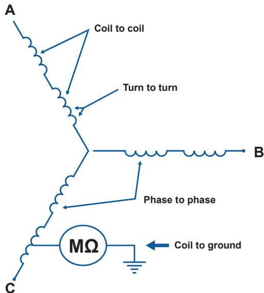
Failures can start between turns in the same coil, between coils in the same phase, and phase to phase. Motor Circuit Analysis using ALL-TEST Pro instruments provides a complete view of the motor in just minutes.
