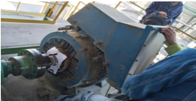
The plant's condition monitoring cell called Prescon for condition assessment of the motor. Prescon utilized ESA (electrical signature analysis) to assess the condition of the motor. Within minutes the test showed that the motor had cracked rotor bars/ end ring problems.
