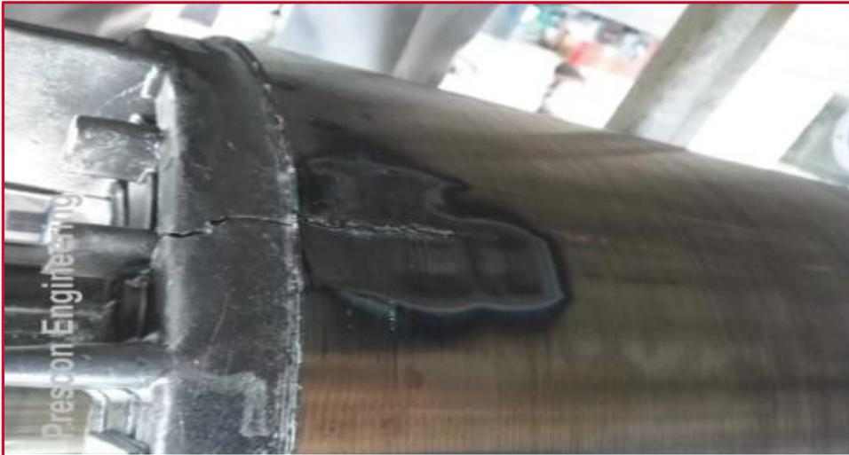
*ESA Technology being used. End ring damage on rotor. Diagnosis was determined after several bearing changes, strange motor behavior and motor trips. Vibration equipment indicated amplitudes that increased and decreased over time between repeated bearing replacement and service intervals. Subsequently the motor was retested with ESA equipment. The problem was not with the bearings but rather the condition of the rotor.*
