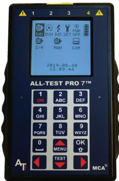
By adding MCA™ readings to DC motor testing provides early indication of developing problems within the motors electrical system beyond those detected using a megohm and ohm meter. MCA tests can be performed quickly from the drive and can confirm or eliminate faults in DC machines.
