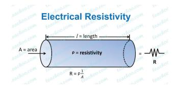
**Conductors** are materials that have loosely bonded electrons in the outer most shell of the atoms making up the conductive material and offer very little resistance to current flow. Electrons flow easily through conductive material. Examples of conductors are copper, steel, iron, bronze, and many other metals.
