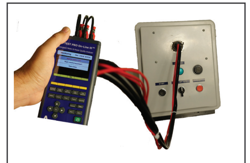
Installed ALL-SAFE inside starter box, connected to ATPOL III™ to start taking readings.
